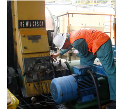
Vibration measurement at a Ball Mill drive
