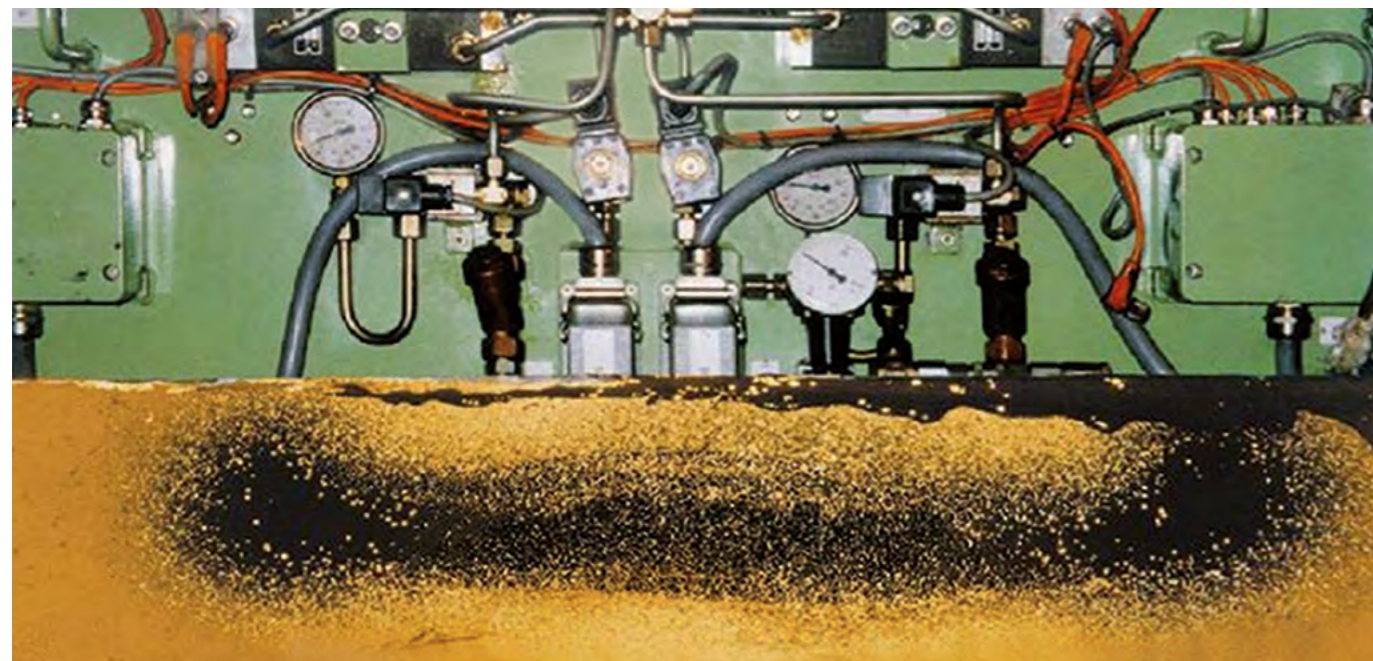
Spray pattern of Berulit on the control panel of a Woerner system
