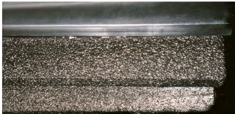
Berulit 443 in a sufficiently strong layer on the flanks
