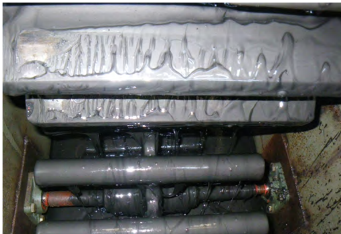
Open Gear drive with paddle wheel lubricated by Berulit GA 2500 Fluid
